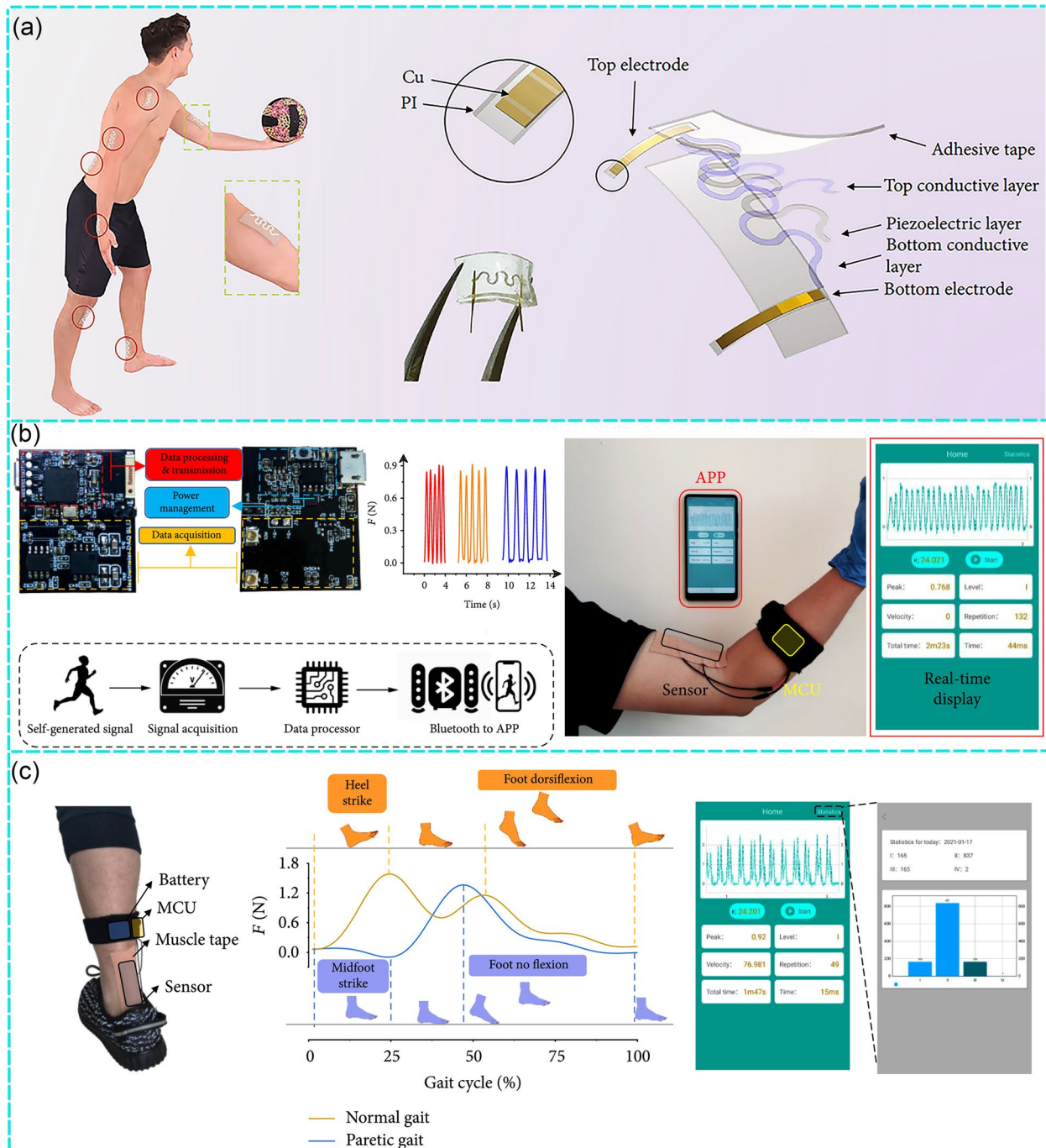
Fig. 4 Applications and an exploded view of the patch (a). The operating procedures of the system and demonstration of applying the patch for recoding the arm's bending (b). An optical image of the patch's fixation, using the bioelectronic system for gait analysis, and APP displays on a cellphone (c). Reproduced with permission from [90]. Copyright © 2021 Sheng Shu et al.
